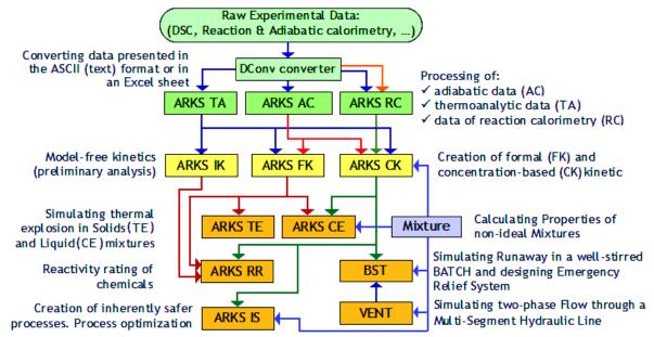
The programs of **the 1<sup>st</sup> group** support all the necessary procedures for proper preparing of adiabatic and thermoanalytical data for kinetics evaluation.
