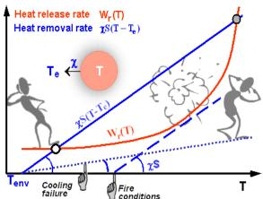
The well-know Semenov diagram demonstrates vividly what the origins of thermal hazard are.
